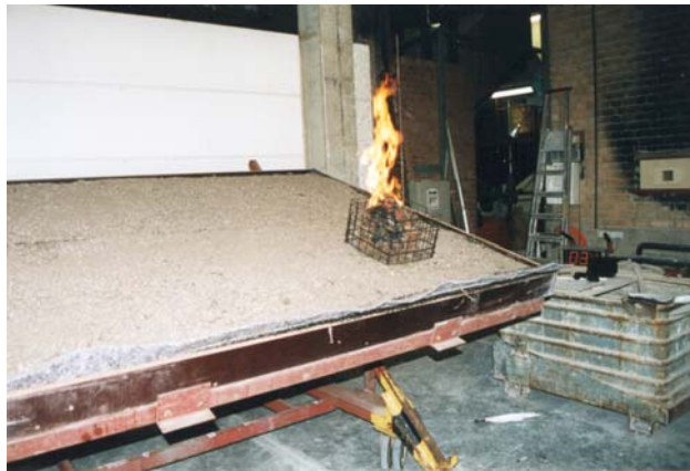
Figure 1: Appearance of the sample roof (15 degrees inclination) during execution of the test.
