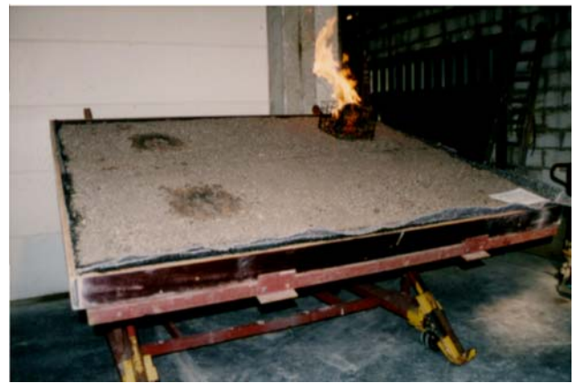
Figure 1: Appearance of the sample roof (15 degrees inclination) during execution of the test.
